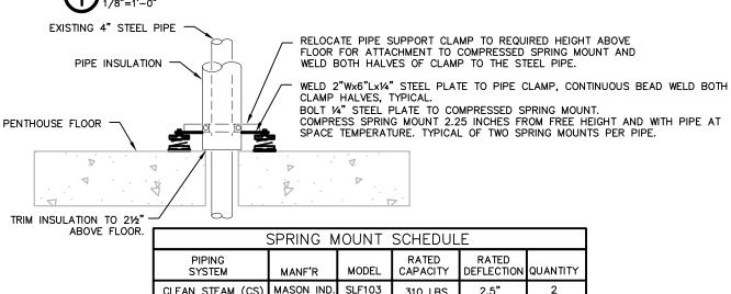
2.5" CLEAN STEAM (CS) 310 LBS. HEATING WATER MASON IND. **SLF104** 500 LBS. 2.5" 2 SUPPLY (HWS) HEATING WATER MASON IND. SLF104 500 LBS. 2.5" 2 RETURN (HWR)
