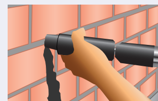
Step 3: Drive the Spira-Lok™ Wall Tie until the nose of the dry set installation tool is hard against the veneer.
